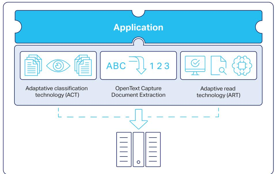
OpenText Capture Document Reader utilizes a combination of rule-based and self-learning modules with the workload distributed over a server cluster. It integrates with third-party applications through an XML interface.
