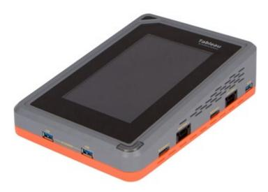
TX1 can operate as a standalone device, as shown above.
