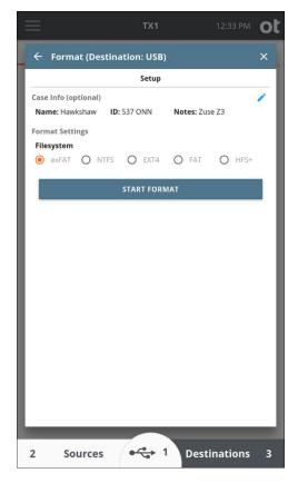
**Note:** TX1 cannot format a destination drive with an APFS filesystem, though it can mount a previously formatted APFS volume on any connected drive (source, destination, or accessory port).
