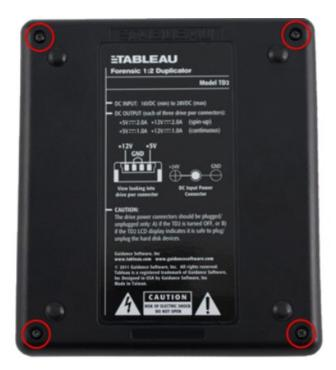
4. If possible, hold the TD2u with one hand as shown in the pictures below. Hold one of the 3M power connectors one each side. This will allow the PCB (Printed Circuit Board) to stay with the top of the case when the bottom is removed.
