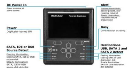
The **SATA Source**, **IDE Source**, and **USB Source** LEDs indicate that the source drive is connected to the left side of the TD2u The **SATA**, **Dest 1**, **SATA Dest 2**, and **USB Dest** LEDs indicate that the destination drives are connected to the right side. A yellow Alert LED on the right flashes to indicate the need for user intervention.
