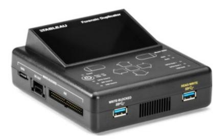
The center button on the arrow keypad also serves as a **[Select]** button when navigating among TD2u menus. It cannot be used to start major tasks, such as duplication or disk wiping. Only soft keys labeled **[Select]** or **[Start]** initiate major tasks. Vertical Arrow Keys scroll up or down and highlight menu items for selection. Horizontal Arrow Keys scroll left or right and toggle between character lists.
