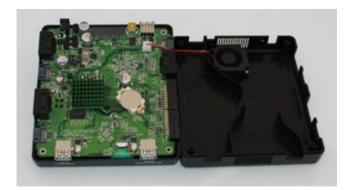
The backup battery is near the heatsink, as shown in the photograph below.
