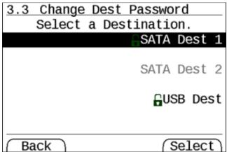
This menu allows you to change the destination encryption header on an already unlocked destination. This does not change the encryption across the drive. Generating a new secure header takes 15 to 20 seconds.
