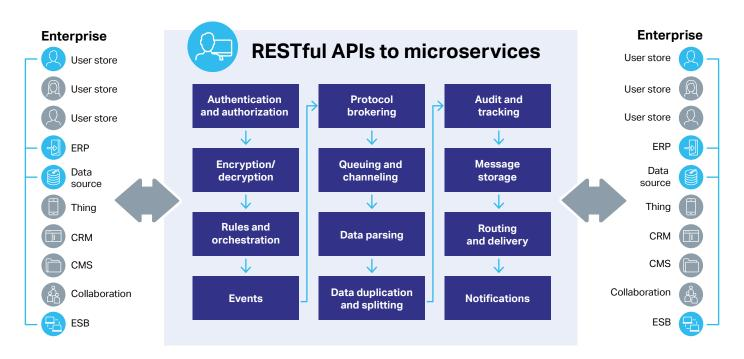
The above diagram highlights a simple enterprise integration use case and sample capabilities. Once the integration endpoint is set up, customers can manage integrations and track messages and failures.
