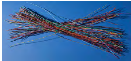
Figure 3.2: According to Grace Hopper, a nanosecond is 11.8 inches long.
