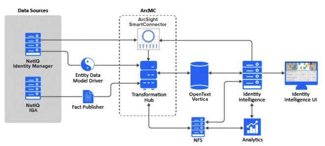
The Identity Intelligence architecture is based on the OpenText<sup>™</sup> Vertica<sup>™</sup> analytical database. This ensures high performance when creating analytical reports, through optimal use of computing resources.
